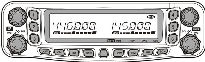
The **FT-8900R** is a ruggedly-built, high quality Quad Band FM transceiver providing 50 Watts of power output on the 29/50/144 MHz Amateur bands and 35 Watts on the 430 MHz band.
