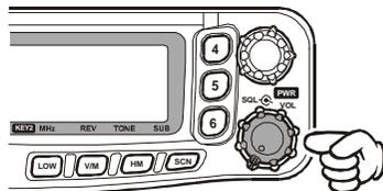
2. To turn the transceiver off, again press and hold in the "right" **VOL** knob for 2 seconds.
