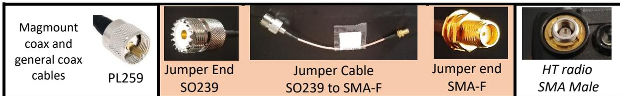
This jumper cable lets us connect an HT to all base station antennas and mobile magmount antennas. Access to the better antennas can improve overall HT performance. There are adapters that attach directly to the HT SMA-M fitting. We prefer to use a jumper cable. We feel this greatly reduces the strain on the radio connector from the weight of any length of RG58, RG8X and RG8/U coax. 🌱
