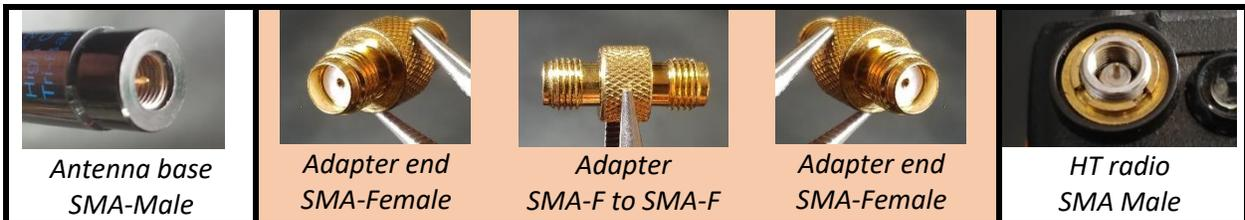
To use the JT-776SMA Tri-band antenna on a mini-magmount for mobile operations, we need to use two additional connectors: 1) an SMA-F to SMA-F to connect the antenna to the Magmount base; 2) an RPSMA-F to SMA-F to connect the coax to the HT. This antenna option will only be considered as an emergency set up if no other antennas were not available. 🌱
