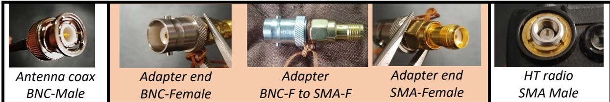
GECO acquired the JT-776SMA Tri-band with a SMA-Male connector, we needed an SMA-F to SMA-F connector to use it with our HT radios.
